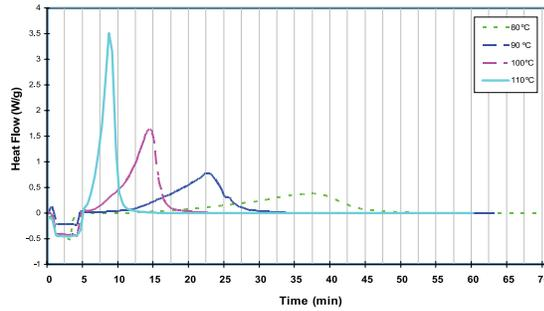
Different exotherm peaks for a typical epoxy at 80°C, 90°C, 100°C and 110°C.
